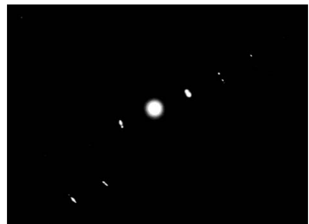
Figure 5 (a) TEM image of a deformation band showing that these bands consists of two, almost parallel walls of high dislocation density, in between which some more dislocations are accumulated. (b) Diffraction pattern of a deformation band and its surrounding area, revealing that the lattice inside the deformation band is rotated by approximately 5°.
